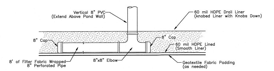
E Leak Detection Detail
